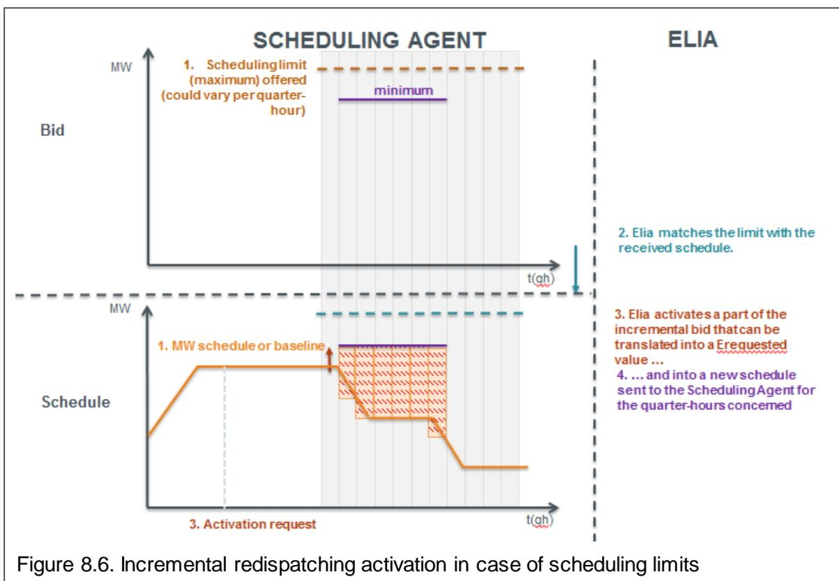
Figure 8.6. Incremental redispatching activation in case of scheduling limits
