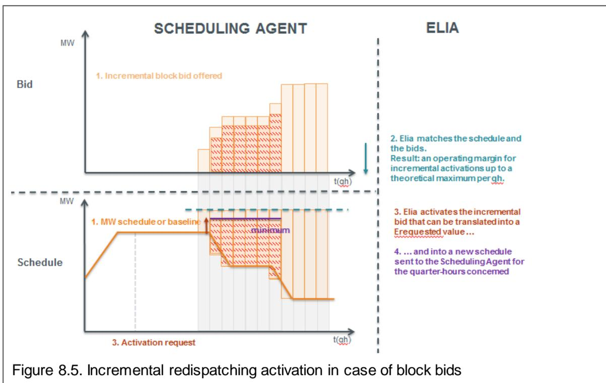
Figure 8.5. Incremental redispatching activation in case of block bids
