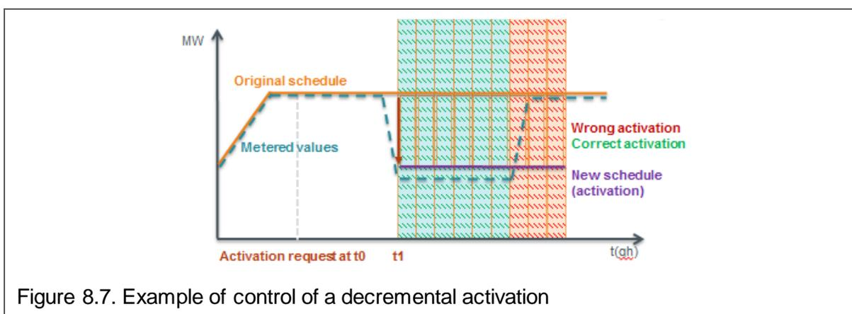
Figure 8.7. Example of control of a decremental activation
